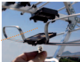
The box is detachable for easy connection of the coaxial cable
